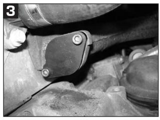
Clean up the face on the exhaust manifold and fit the new blanking plate using the existing pins and some exhaust assembly paste if needed.
