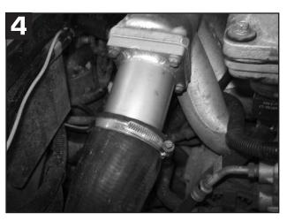
Clean surface of inlet manifold, fit gasket and new inlet adaptor then secure with original fixing bolts. Remove rag from hose and refit to adapter and tighten jubilee clip.
