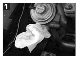
Remove sound deadening pad of the engine and top radiator cover, also if needed, remove engine fan to allow easy access.
