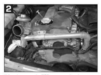
If fitted remove the EGR water cooler pipes, re-route them down the side of the engine and join them together and secure them to the engine.
