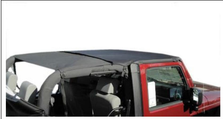
10. Wrap the straps at the rear corners of the top around the roll bar and tighten.
