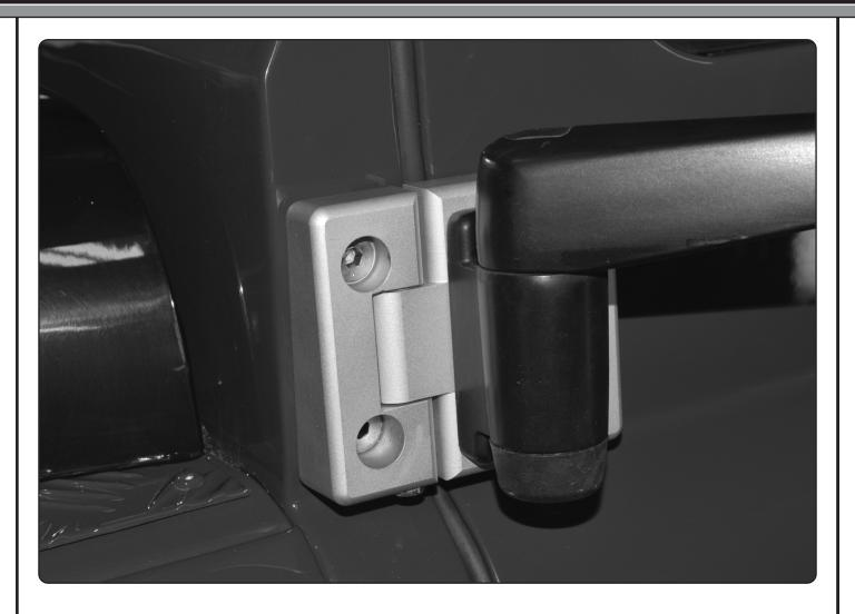
Bolts are left long to accommodate extra packing pieces if necessary. If extra packing is not required the bolts may need trimming back to clear the door card. This will be best done after the nuts have been tightened.
