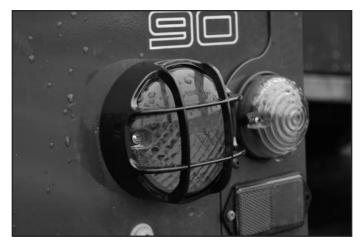
These guards will fit all of the 95mm diameter lights used on Defenders - fog, reverse and also NAS spec lights.
