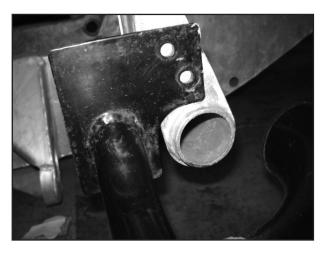
Use an 8.5mm drill bit to drill the holes and remove any sharp edges with a file.
