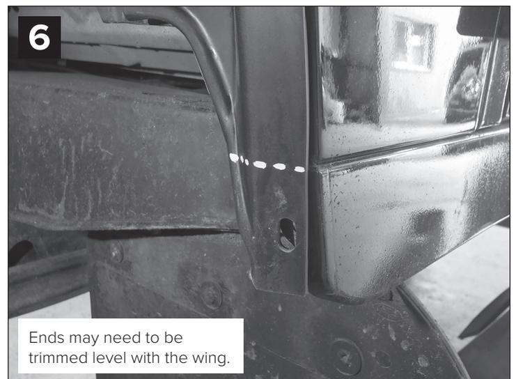
**Last Stage** - First hold arch in position then the fill in piece, line holes up and fix in place. Starting from centre top working your way down either side.
