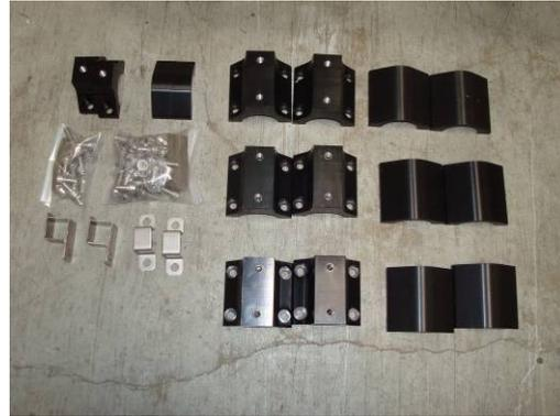
1.4 - The aluminium clamps and stainless brackets need to have the self adhesive rubbers applied to them at this stage.
