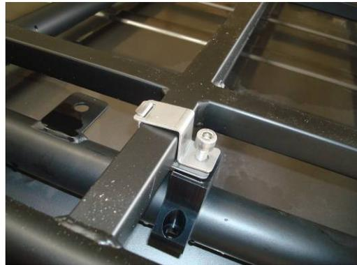
2.4 - Using the M8 x 16mm countersunk bolts and spring washers provided, attach the lower section of each clamp to the upper section. Copper grease should be applied to the threads to aid fitment. These should not be tightened fully at this stage.
