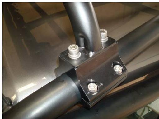
2.5 - All bolts can now be gradually tightened to **25Nm** ensuring that the rack sits position does not change whilst working around the vehicle.
