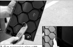
3. Cut excessive pins with sharp knife
